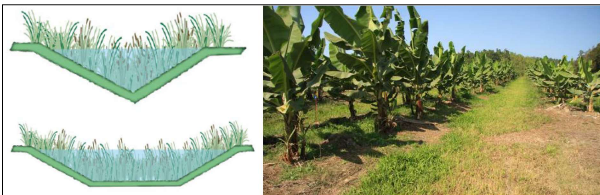
Figure 6: Left: Diagram to show cross sections of vegetated drains (top) and vegetated swales (bottom). Right: Example of a wide, vegetated spoon swale on a banana property (Source: Queensland Department of Environment and Science, WetlandInfo 2018b).
